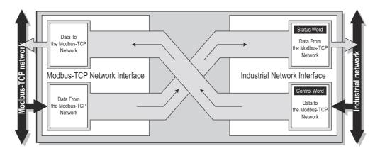
Each buffer holds a maximum of 256 bytes of data. The first two bytes in either direction can be dedicated for control/status information, and another eight bytes of data coming from the Modbus-TCP network can feature a live list. Please note that the actual number of bytes that can be exchanged is highly network dependent.
