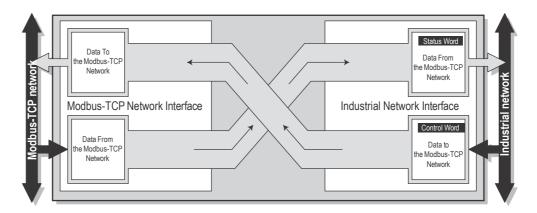
Each buffer holds a maximum of 256 bytes of data. The first two I/O mapped bytes in either direction can be dedicated for control/status information, and another eight bytes of data coming from the Modbus-TCP network can feature a live list. Please note that the actual number of bytes that can be exchanged is highly network dependent.
