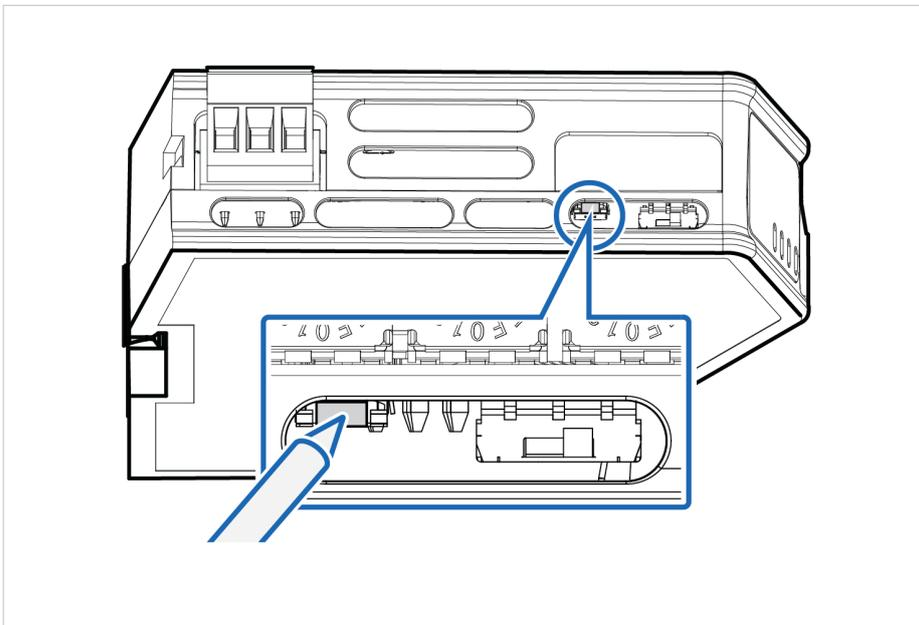
Figure 46. Press and hold **Reset** button
