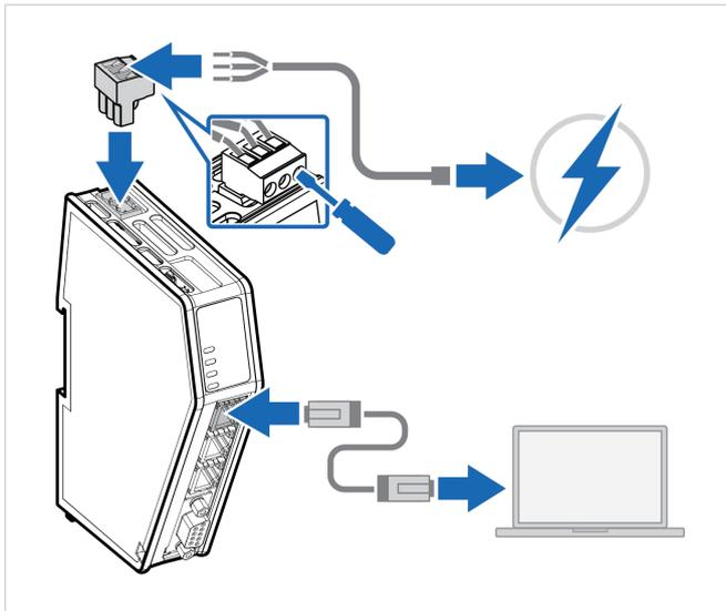
1. Connect an Ethernet cable between the Communicator and your PC.
