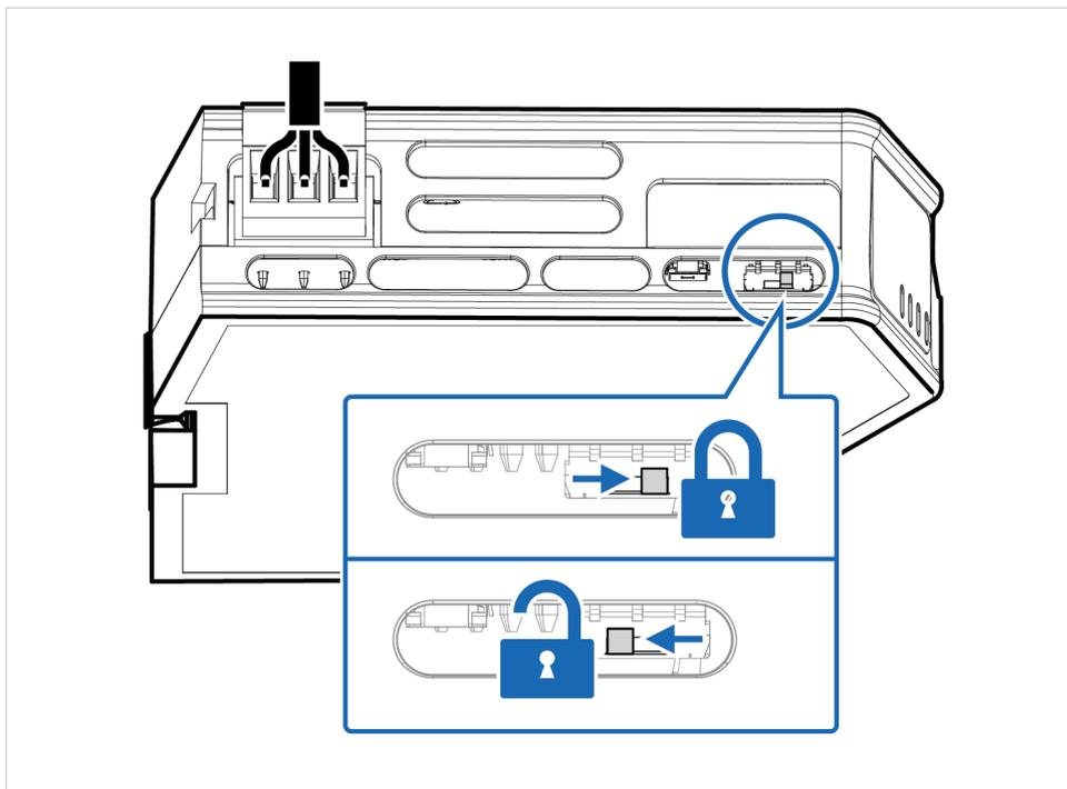
Figure 11. Security switch in locked and unlocked position
