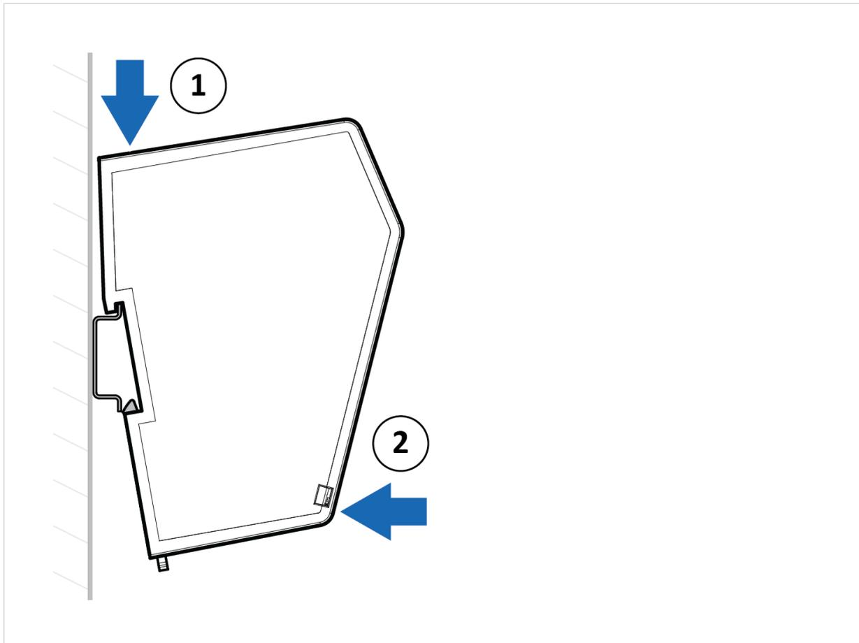
Figure 4. Attach the Communicator on the DIN rail
