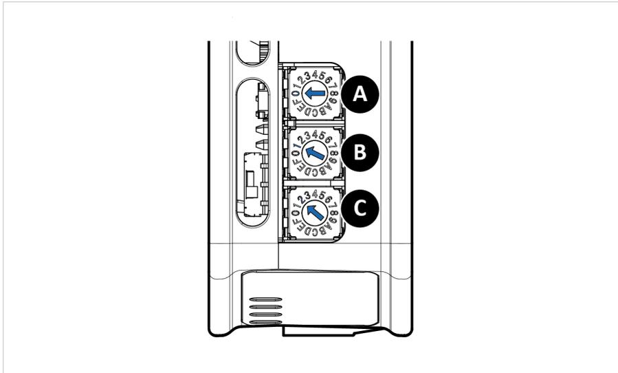
1. The rear rotary switch A is not used, ensure that it is set to 0.
