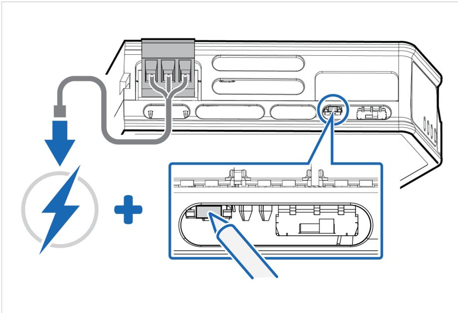
Figure 47. Hold **Reset** button and reconnect power
