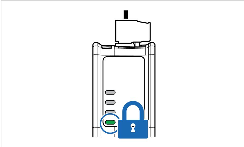
Figure 12. Security switch locked status LED
