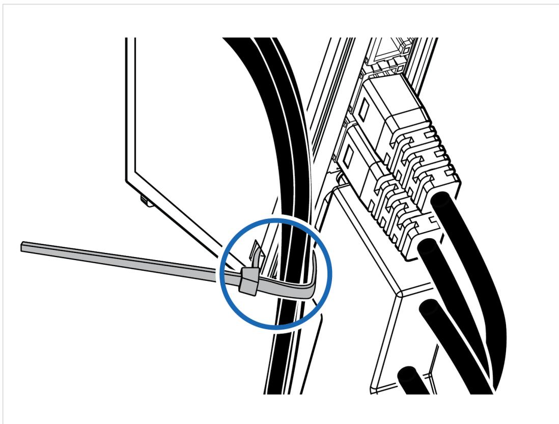
Figure 13. Lock the cables
