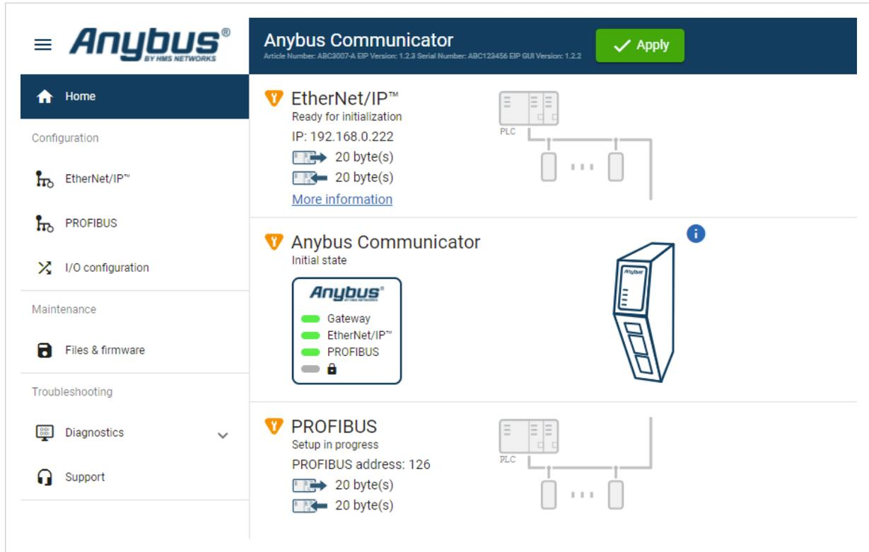
Figure 16. The Communicator built-in web interface Home page
