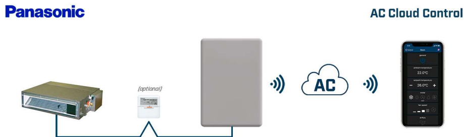
Use Case Integration of Panasonic ECOi & PACi systems into AC Cloud Control.
