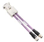
Where slave device uses M12 connectors, use the Procentec DB9-M12 Tap Lead (with part no. 101-00052B – as in photo) or similar. The Procentec assembly includes both male and female M12 connectors and allows connection onto the HP-25 tester. Note that the two short M12 connection leads are joined within the 9-pin connector – ie the terminator switch cannot be used here to isolate test signals from outgoing cable.
