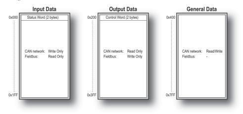
Note 1: The picture shows the maximum available data areas in the Communicator. Not all fieldbuses can access all addresses in the input and output data areas, please see section Data Exchange Model in chapter 1.
